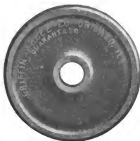
Figs. 4547-4548. 700-lb. Double Plate Cast Iron Wheel. Griffin Wheel Co.
